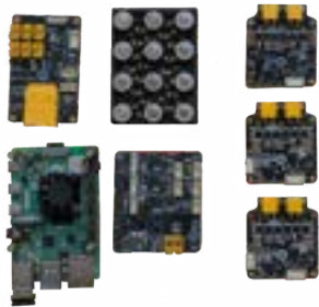
Electronics: Rpi, Power Distribution board and motor controllers
