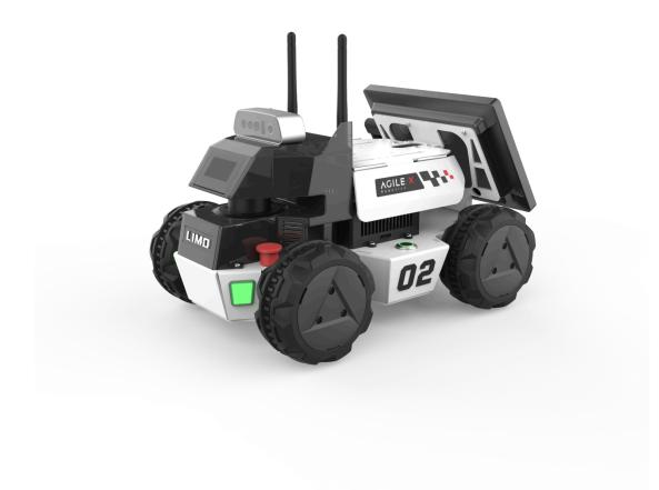
**LIMO ROS2** robot features an Intel NCU i7 processor running ROS 2 on Ubuntu 22.04, providing an essential platform for autonomous mobile robot research and education.
