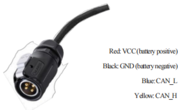
Figure 3.2 Schematic diagram of the male aviation plug
