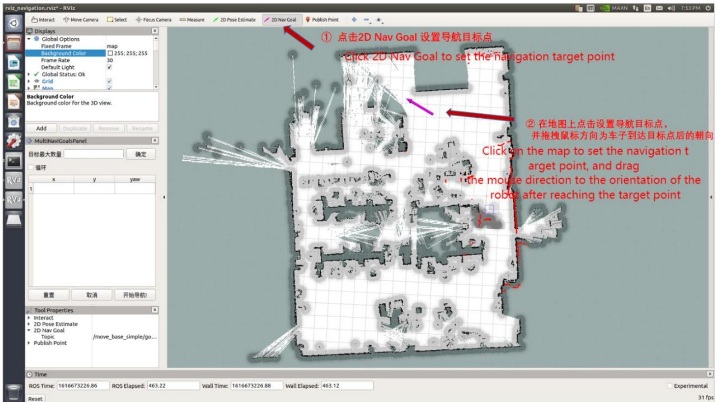
已生成目标点The target point has been generated.
