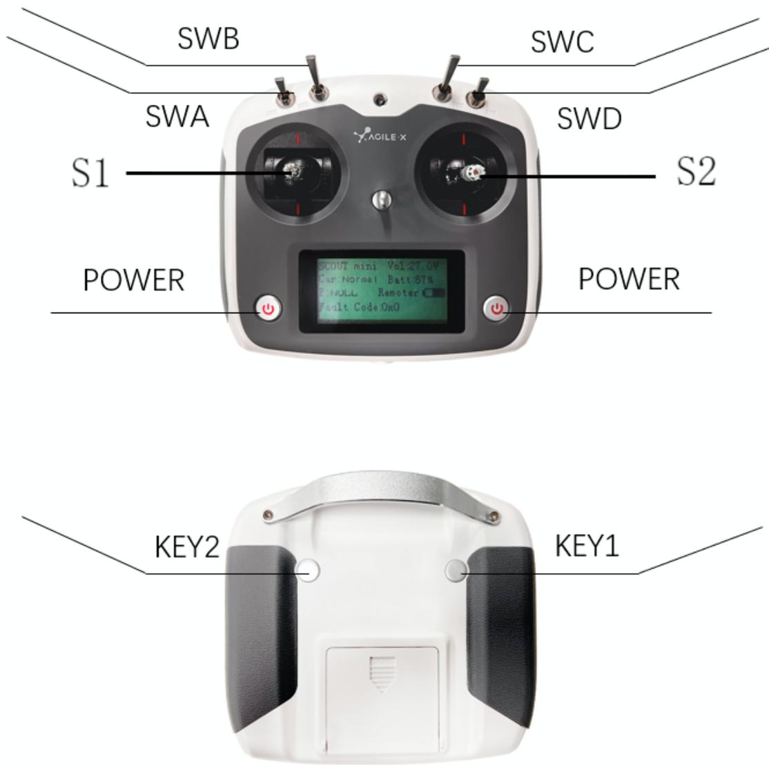
Figure 2.3 Schematic diagram of FS remote control buttons
